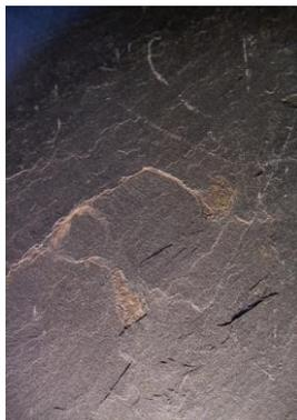
A close-up showing how a pyrite has oxidised and spread within the slate's structure.
